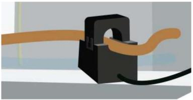
5. Plug the end of the clamp cable into input 1 of the Smappee monitor.
