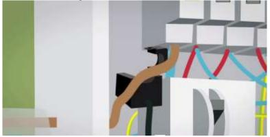
8. Plug the cable of the second clamp cable to input 2 of the Smappee monitor.
