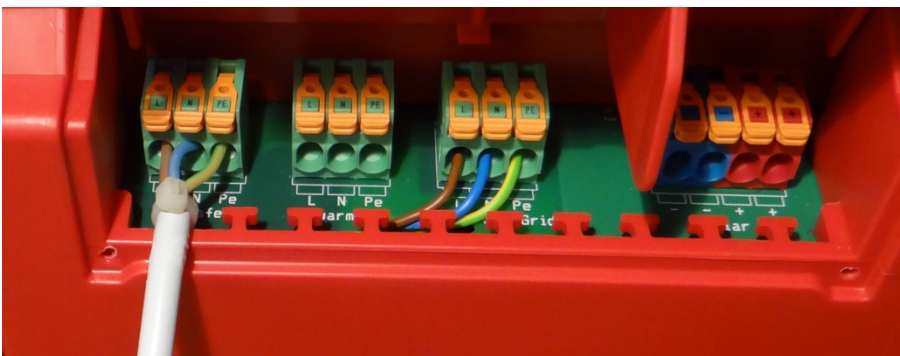
Figure 12: Securing the cable with a cable tie on the strain relief bar
