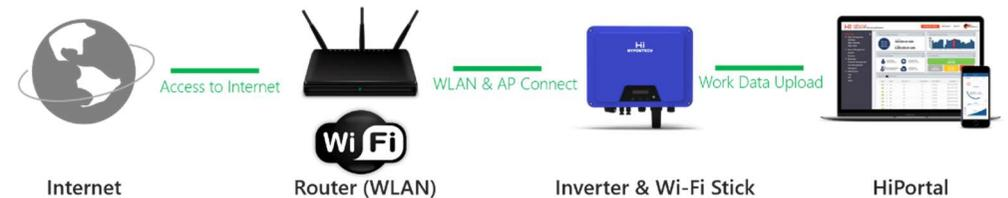
Uploaded data from the inverter are displayed on HiPortal once it is added to a PV plant.
