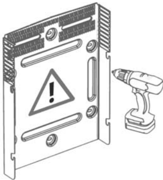
Figure 2.10 : Montage du support mural
