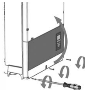
Figure 2.15 Loosen front screws and lift the cover
